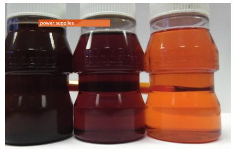
Above: Fuel held within back-up generators can sit in tanks for so long it becomes problematic, clogging up generators and causing emergency systems to fail. Fuel polishing systems help to remove dirt and bacteria and return fuel to its original condition Right: WASP PFS fuel cleaning systems are being used by a number of hospitals in the UK, ensuring they have back-up power in
